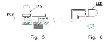
2. Lead forming or bending must be performed before soldering, never during or after soldering.
