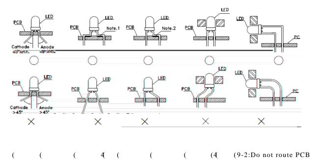
Trace in the contact area between the lead frame and the PCB to prevent short-circuit.
